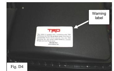
4. Apply TRD air filter warning label to area pre-cleaned from the steps above. (Fig. D4)
